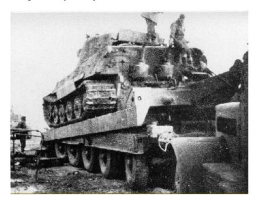
Above: Tiger 121 has been loaded onto the specially constructed trailer. Just visible above the "white box" on the trailer is one of the hydraulic rams that lowered down once the pull had been completed.
